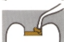
FIG. 15*—Marginal deficiency being corrected by filling the resultant enlarged void.
